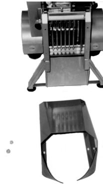
7. Unfasten the Safety-Screw at the right side of the machine. Remove the safety covering and attach the side hopper at this point.
