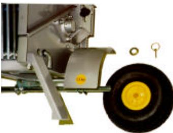
5. Install the feet and the rear tunnel at the cutting-unit side of the machine. Do not forget to install the cross-beam between the feet.
