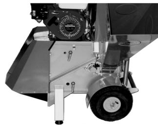
8. Put the square spanner for tensing the v-belt in the holding fixture at the right side.
