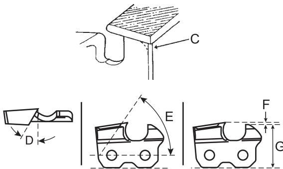
5. Finish cutter sharpening by rounding front raker edge (C) with flat file.
