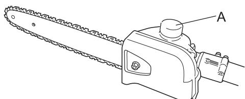
1. Place the unit on a clean, flat surface with the oil filler cap (A) facing up. Wipe off any debris from the oil cap and from around the oil filler neck.
