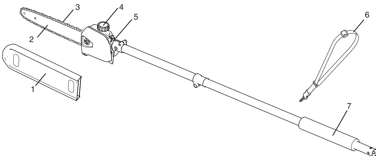
1. **Guide bar cover** - Used to cover guide bar and saw chain during transport and storage. Remove guide bar cover before using unit.
