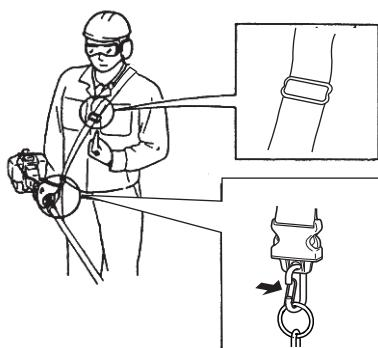
1. Hook the strap hook to the hanger on the outer tube.
