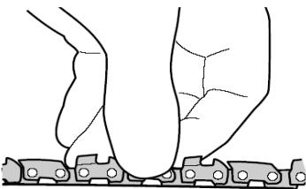
4. Pull the chain by hand along the top of the guide bar several times from the motor to the bar's tip. The chain should feel snug but still pull freely.
