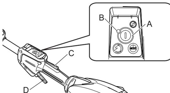
1. Release trigger switch and trigger switch lockout, and allow the attachment head to stop.
