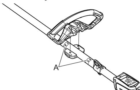
Position handle in comfortable operating position and tighten Bolts.
