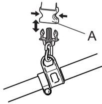
1. Hook the strap hook to the hanger on the outer tube.
