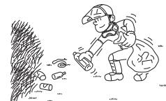
An accident or serious injury can occur if foreign objects ricochet off the cutting attachment or wire and other materials twisted round the product spring off it.
