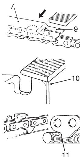
When setting of the chain is finished, soak it in oil and wash away filings completely before using.
