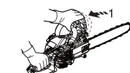
♦ Squeeze throttle trigger gradually to increase engine revolution.
