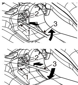
1. Spark plug cover      2. Spark plug cover latch      3. T-wrench
