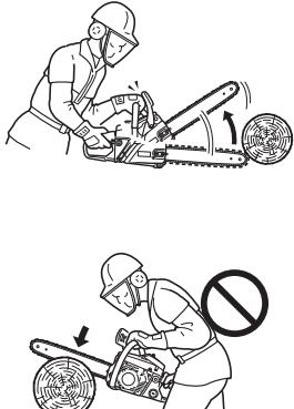
The chain brake's function is to stop chain rotation after a kickback.
