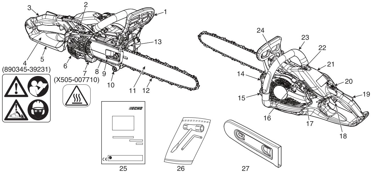
1. **Front hand guard** - Guard between the front handle and the saw chain for protecting the hand from injuries and aiding in control of the chain saw if the hand slips off the handle.
