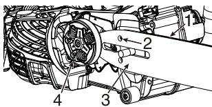
1. Groove      2. Oil hole      3. Guide bar      4. Sprocket
