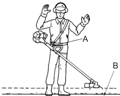
Balance tool for a level plane of cutting head rotation
