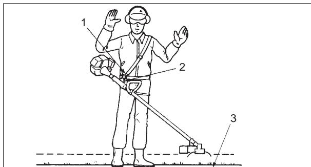
**Balance tool for a level plane of cutting head rotation** 1. Harness quick-release pin
