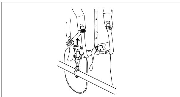
Place shoulder harness over both shoulders and adjust straps so the connecting point latch as shown.
