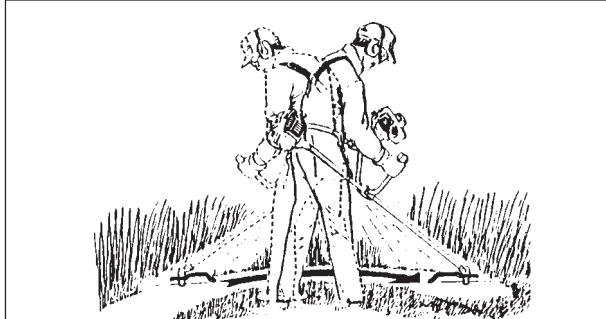
**SCYTHING WEEDS.** This is cutting by swinging the cutting attachment in a level arc. It can quickly clear areas of field grass and weeds. Scything should not be used to cut large, tough weeds or woody growths.
