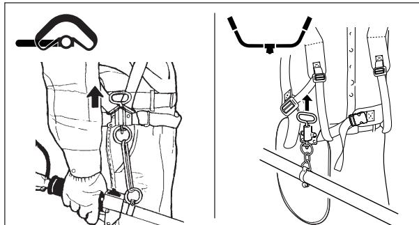
Place shoulder harness over left shoulder and adjust straps so the quick-release pin rests just below the waist.
