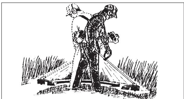
**SCYTHING:** This is the cutting or mowing of large grassy areas by sweeping or swinging the trimmer in a level arc. Use a smooth, easy motion. Do not try to hack or chop down the grass. Tilt the line head or line disc to direct the debris away from you on the scything stroke. Then return without cutting grass for another stroke. If you are well protected and do not care whether some debris is thrown in your direction, you may scythe in both directions.
