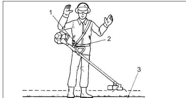
Balance tool for a level plane of cutting head
