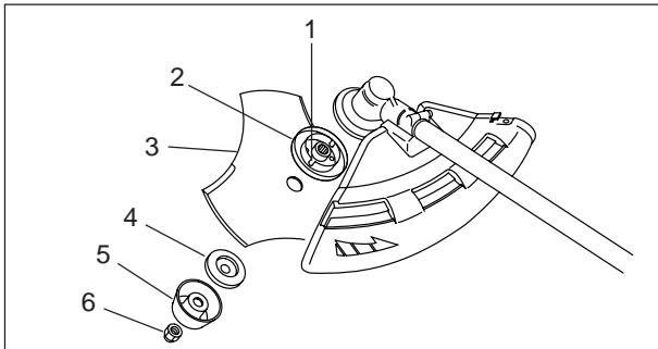
1. Blade retainer fixing slot    4. Lower blade retainer
