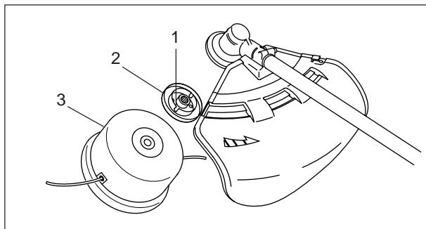
1. Blade retainer fixing slot
