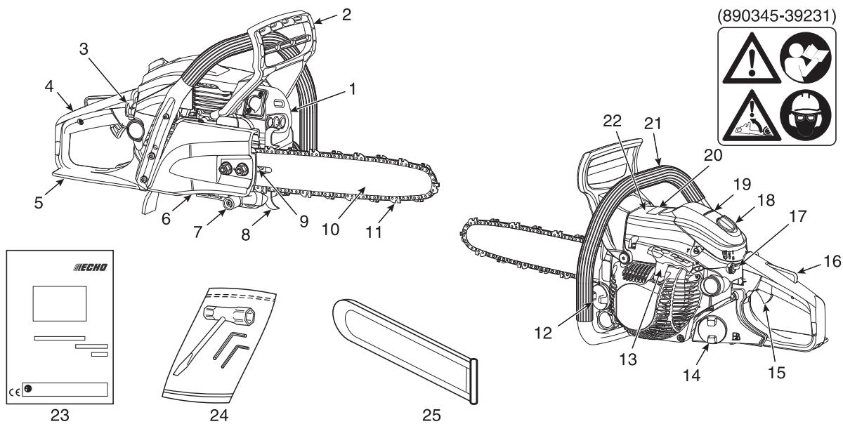
1. **Silencer** - The silencer controls the exhaust noise and prevents hot, glowing particles of carbon from leaving the silencer.
