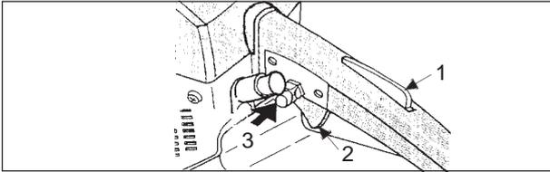
1. Throttle trigger lockout
