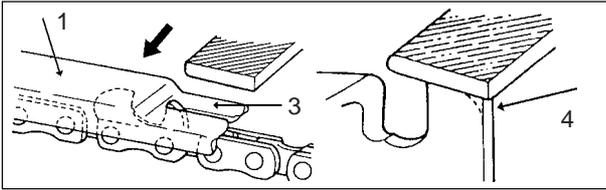
1. The depth control determines the thickness of wood chip produced and must be maintained correctly throughout the chain life.
