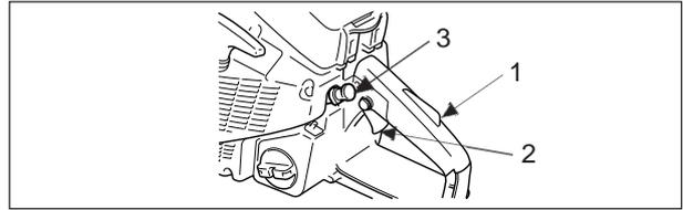
1. Throttle trigger lockout
