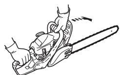
1. Place the chain saw on the ground.
