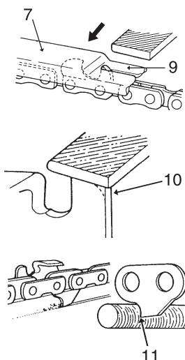
When setting of the chain is finished, soak it in oil and wash away filings completely before using.
