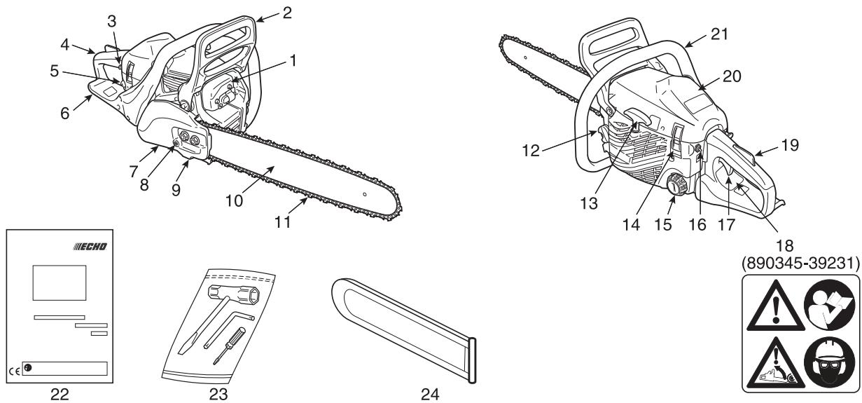
1. **Silencer** - The silencer controls the exhaust noise and prevents hot, glowing particles of carbon from leaving the silencer.
