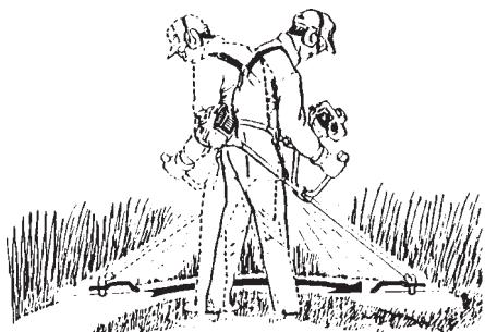
**SCYTHING WEEDS.** This is cutting by swinging the cutting attachment in a level arc. It can quickly clear areas of field grass and weeds. Scything should not be used to cut large, tough weeds or woody growths.
