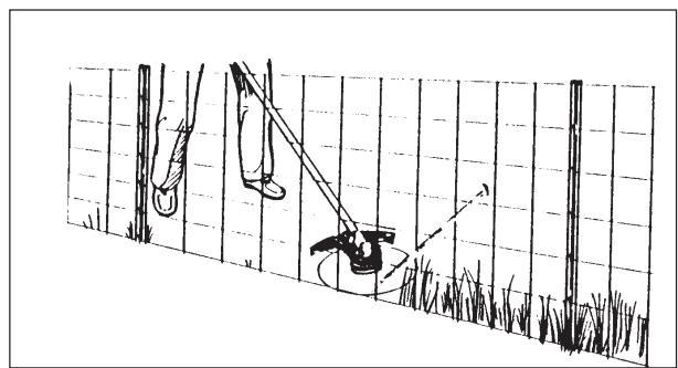
Always wear proper eye protection against thrown objects. Objects can bounce up at you from the ground under the shield, or ricochet off any nearby hard surface.
