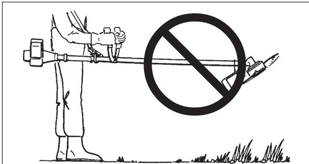
Do not raise the cutting attachment above knee height. If raised higher, the cutting attachment will be more directly in line with your face. Thrown objects may hit your face and eyes.
