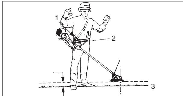
**Balance tool for a level plane of cutting head rotation**
