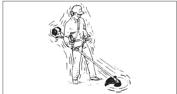
Stop the engine before leaving the machine, children are not allowed to use the machine with metal tools, stop the machine between different working places.
