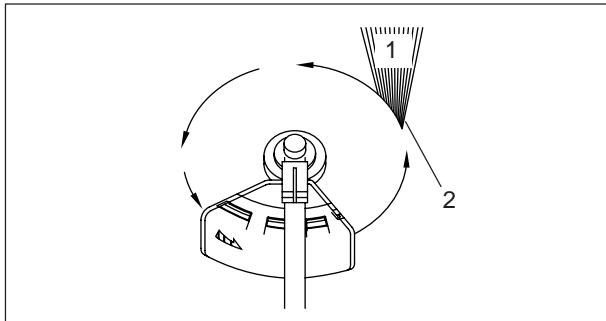
**Nylon line head or disc rotates anticlockwise.
