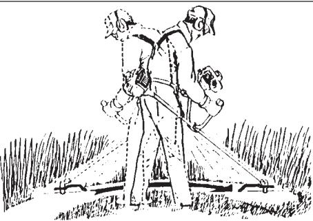
**SCYTHING:** This is the cutting or mowing of large grassy areas by sweeping or swinging the trimmer in a level arc. Use a smooth, easy motion. Do not try to hack or chop down the grass. Tilt the line head or line disc to direct the debris away from you on the scything stroke. Then return without cutting grass for another stroke. If you are well protected and do not care whether some debris is thrown in your direction, you may scythe in both directions.
